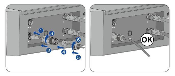
**Step 5:** Connect the terminating resistor to the "Link Port Out" of the BCU.
