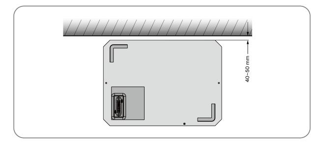
**Step 3:** Remove a battery module from the package. Place one battery module on the base and secure the battery module by the supplied screws(M5×25). Tightening torque: 4 Nm. Pay attention to the direction of the module. The power-mating connectors on the battery module and the base should be on the same side.
