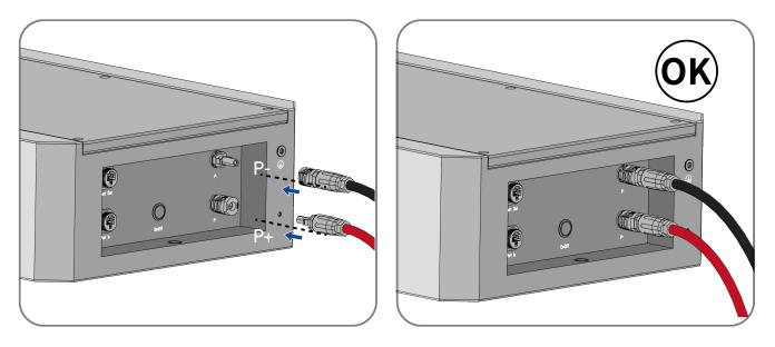
**Step 2:** Add the connector from the inverter package to the opposite ends of the power cables and connect them to the inverter battery input connectors.
